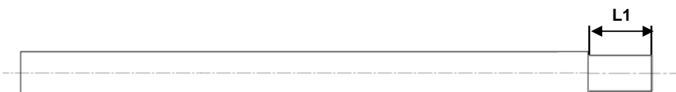
Figure 30: Stripping length L1
