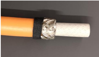
Figure 41: Fold over and fix the shielding
