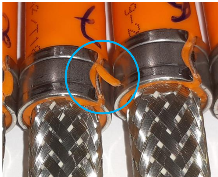
Figure 40: Scraping during cimp-process
