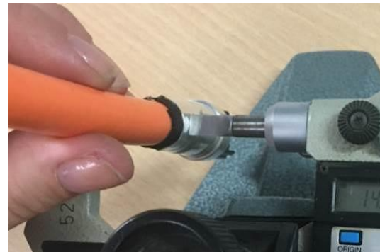
Figure 60: schematic representation of the pressing height measurement
