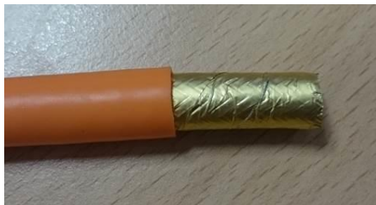
Figure 29: Strip off shielded cable
