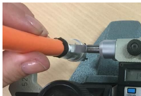
Figure 68: schematic representation of the measurement of the pressing height
