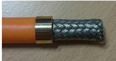
Figure 32: remove the foil
