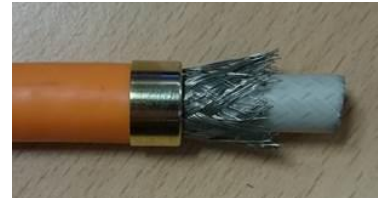
Figure 33: shorten the shielding
