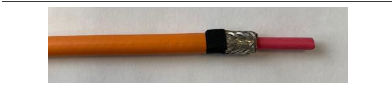
Figure 3.17: Representation 4.0 mm 2 SCC position fixing tape related to the ferrule crimp (3.5 Fold over the shielding braid and secure the shielding braid)
