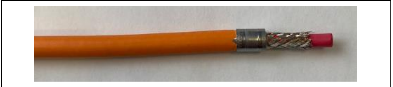
Figure 3.7: Representation 4.0 mm 2 SCC remove shielding foil (if present), trim shielding braid, and crimp the ferrule crimp (3.4 Remove shielding foil (if present), trim shielding braid, and crimp the ferrule crimp)
