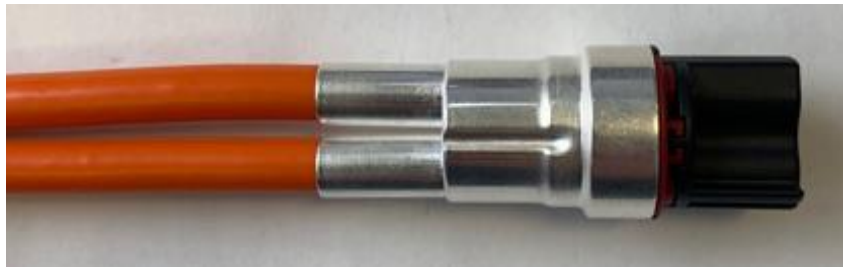
Figure 4.20: Representation 6.0 mm 2 SCC slide the shielding sleeve onto the contact carrier (4.8 Slide the shielding sleeve onto the contact carrier)
