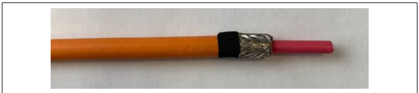
Figure 3.15: Representation 4.0 mm 2 SCC fixing the shielding braid (3.5 Fold over the shielding braid and secure the shielding braid)
