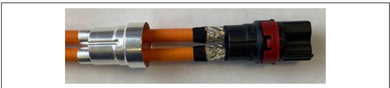
Figure 3.34: Representation 4.0 mm 2 SCC protruded individual shielding strands (3.9 Slide the shielding sleeve onto the contact carrier)
