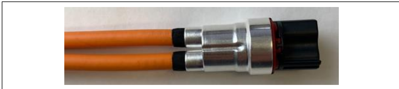
Figure 3.29: Representation 4.0 mm 2 SCC slide the shielding sleeve onto the contact carrier (3.9 Slide the shielding sleeve onto the contact carrier)
