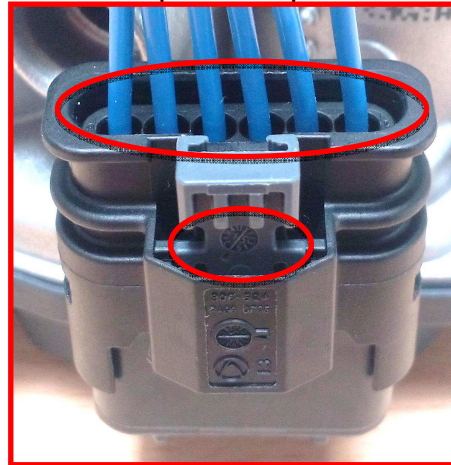
female housing + protective shroud + CPA in pre-lock position
