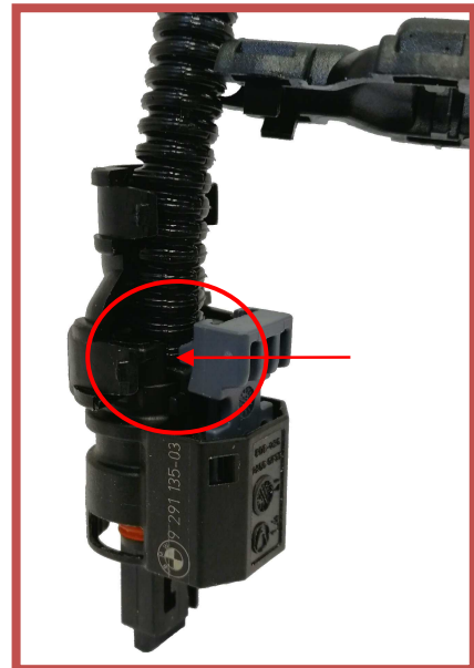
The corrugated pipe must not blocking the traversing distance of contact housing.
