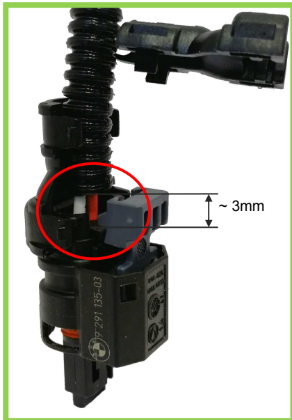
Between corrugated pipe and contact housing has to be a minimum distance of 3mm.
