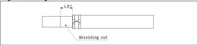
Depending on the production method of each manufacturer, the dimension L5 can vary. After cutting the shield, there are no wire residues or parts of the shielding allowed on the cable. This must be ensured with actions like the following:
