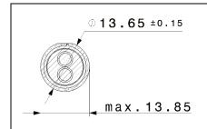
When pressing the ferrule crimp, the dimension is  $\emptyset 13.65 \pm 0.15$ .
