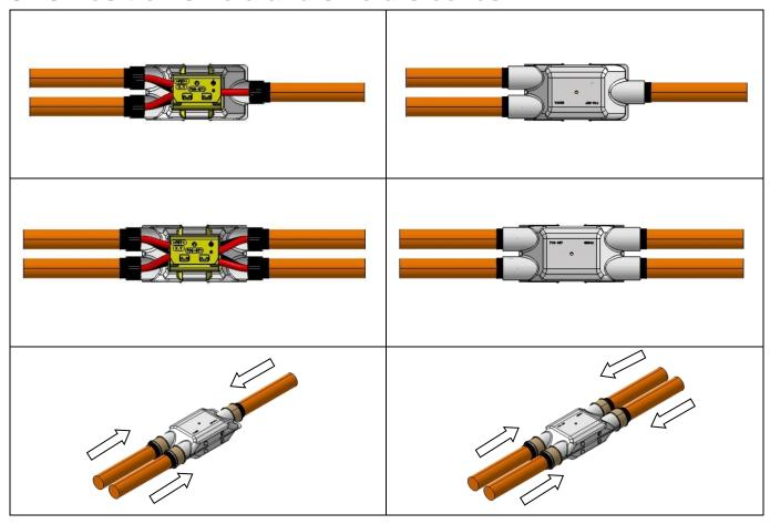
The shield consists of two identical parts. The isolator is positioned within the shield. If the isolator is positioned correctly in the first shield, the second shield can be assembled.
