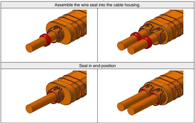
The seal may be expanded slightly during assembly. It may be pushed with the cap, but may not be twisted, jammed, or damaged during this process.
