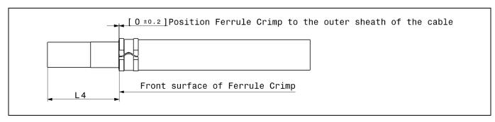
The ferrule crimp must be positioned in relation to the outer jack of the wire. The dimension of [0± 0.2] must be maintain. When the ferrule crimp is crimped on the wire, the insulation can be pushed forward, and the dimension can no longer be maintained. Therefore, dimension L4 should be used as a check. An overlap of the foil in the area of the ferrule crimp like small edges is allowed.
